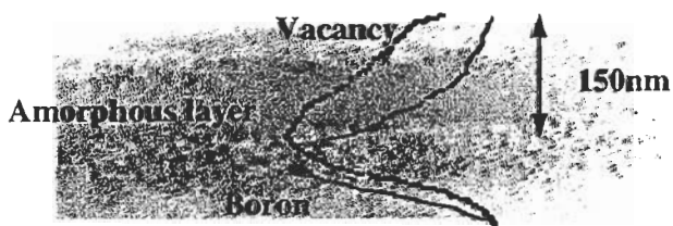
Fig. 4 XTEM bright field image of boron ion implanted silicon wafer with dose of 1 \times 10^{16} ions / \text{cm}^2 .
